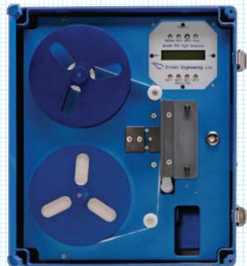
331 Unit with cover removed
