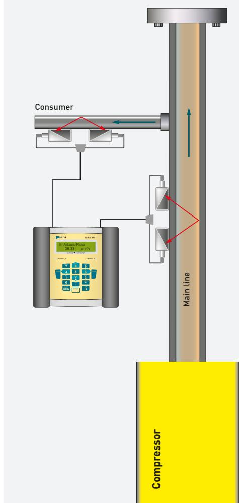
**FLUXUS® G601 CA Energy** is not only capable of measuring the flow rate of liquids, but also thermal energy quantities and flow rates of industrial gases. Thus, the **FLUXUS® G601 CA Energy** has especially been designed for the non-intrusive flow measurement of compressed air.
