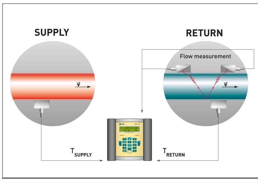
**FLUXUS® F601 Energy** measures the thermal energy consumed by a system by determining the heat or cold flows entering and exiting it (difference method). For doing so, temperature measurements at the supply and return lines as well as the measurement of the volume flow through the system are required. **FLUXUS®** uses the measured values to calculate the thermal energy flow based on the heat transfer media's enthalpy curves stored in the internal memory.
