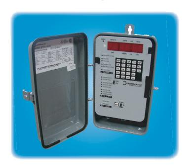
The M-415 Signal Controller is a fully enclosed, electronic device which provides for programming and control of 7 day or full year timed signals. A solid state time switch permits 1000 ON/OFF set points on independent daily schedules through a 7 day time period and across 99 separate holiday schedules. A factory installed field replaceable lithium battery maintains accurate time keeping and calendar information for a minimum of 8 years.
